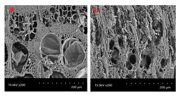
**Figure 1.** SEM microphotography of anatomical elements of wood: (**a**) Fresh-cut; (**b**) archaeological elm wood.
