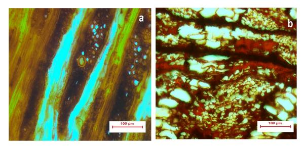
**Figure 2.** Microscopic image of archaeological elm specimens degraded by erosion bacteria: (a) Tangential section; (b) transversal section.
