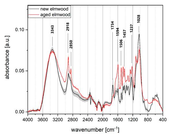
**Figure 3.** FTIR spectra of fresh-cut and archaeological elm wood specimens. The semi-transparent area around the data plot indicates the standard deviation of the two averaged spectra.
