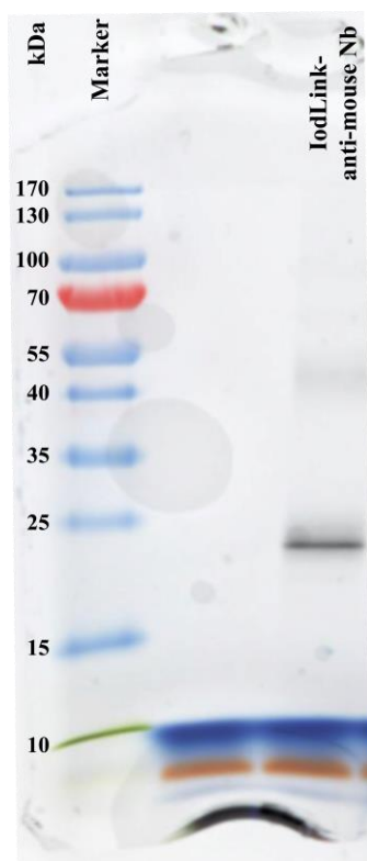
Figure S1. SDS PAGE of IodLink-nanobody anti-mouse IgG after SE-HPLC purification. The expected mass range of ~22 kDa is indicated by the SDS gel. FI-Red: Fluorescence, Epi-RGB (red), light 630 nm, filter Cy5. Marker = PageRuler protein ladder (ThermoScientific, Germany).
