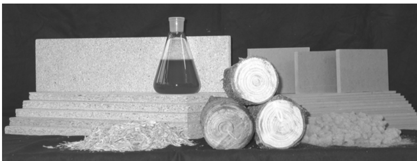
Fig. 2 Wood of low quality can be chipped or disintegrated into fibres, the chips and fibres incubated with a laccase solution (present in the Erlenmeyer flask) to activate the natural bonding forces of lignin in order to subsequently be pressed into particleboards (shown at the left) or medium-dense-fibreboards (MDF), respectively. Further details are given in Chapter 18 of this book. The photo was kindly supplied by C. Schöpfer
