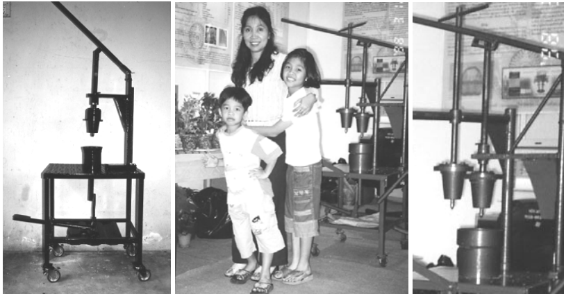
Fig. 9 Manually-operated compactors for the small-scale production of pot plant containers in Thailand
