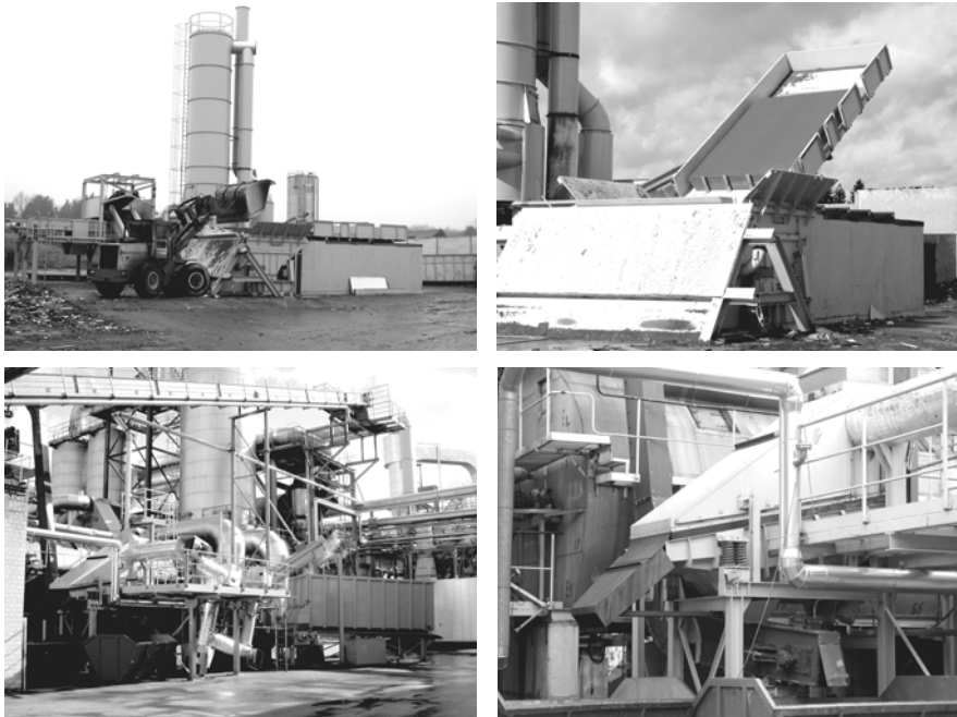
Fig. 4 The thermo-hydrolytic Conti-Recycling-Process developed by the Pfeleiderer Holzwerkstoffe & Co. KG for disintegration of particle boards (Kharazipour et al. 1999, 2000, Kirchner & Kharazipour 2002a,b, Stracke et al. 2001). Wood composites are loaded into a conventional pre-crusher (shown in full view in the upper left photo; loading is shown in the upper right photo). Palm-sized pieces from mechanical chopping in the pre-crusher (see Fig. 5) are subjected in screw conveyors in a disintegration plant (lower left photo: pilot plant at Rheda, Germany) to decomposition in a closed system of saturated vapour typically at a temperature between 120 and 180°C (optimum 140°C). Sorting of the chip material by size into cover and intermediate layer chips for particle production and separation from oversized wood chips, coating remainders and other foreign matter is performed under vibration in a terminal sieving step in a vibro-sieve chamfer-line (shown enlarged in the lower right photo). For further details see Fig. 6
