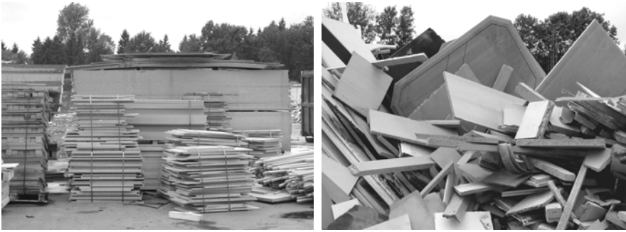
Fig. 1 Rejections of particleboards (left photo) and a heap of board material from discharged furniture and production remainders (right photo) as material for recycling in the panelboard industry
