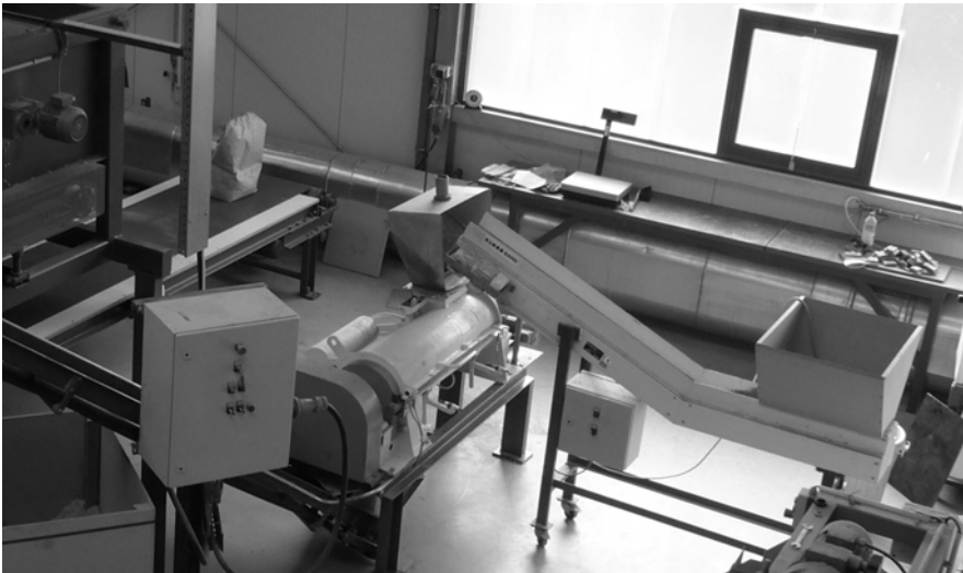
Fig. 19 Pilot plant for particle board production in the “Biotechnikum” at the Institute of Forest Botany in Göttingen. Top: two bunkers in line allow the production of three-layered boards. Bottom: particles are transported via a conveyer belt into the blender (further details in Fig. 20)
