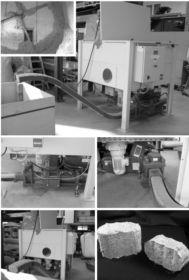
Fig. 8 Briquette machine (full view at the top; top left: view into the dosing bin showing a rotating wheel pushing particles into the inlet of the briquette press; row below: enlarged views of the engine and the outlet of the ready briquettes) in the Biotechnikum (pilot plant station) at the Institute of Forest Botany in Göttingen used to fabricate briquettes from wood waste materials (bottom right; photos by S. Dantz & C. Schöpfer). Research projects on fabrication of briquettes address different lignocellulosic materials, different types of bonding agents, and heating values of resulting products (Vetter et al. 2007)
