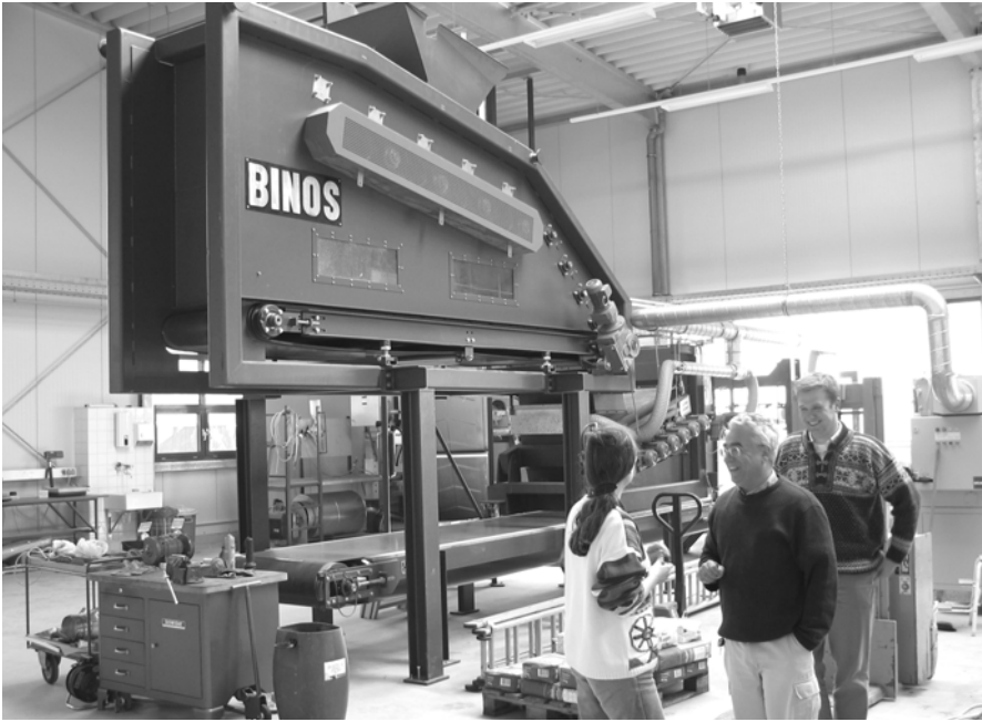
Fig. 16 MDF pilot plant in the “Biotechnikum” at the Institute of Forest Botany in Göttingen. This first fully-automatic pilot plant in Germany was developed and constructed in cooperation with the company BINOS Technologies GmbH & Co. KG (Springe, Germany). The construction and technical equipment matches industrial plants and allows fully-automatic bulking, gluing, drying, and spreading of fibres (see Fig. 17 for further details). The pilot plant can produce fibreboards up to 20 mm in thickness by dry-, semi-dry, and wet-processes. It can be operated with all kinds of fibre material (wood, hemp, flax, straw, etc.) and conventional resins as well as natural binder systems. The pilot plant is used mainly for research on alternative raw materials and new bonding agents and for development of new generations of fibreboards
