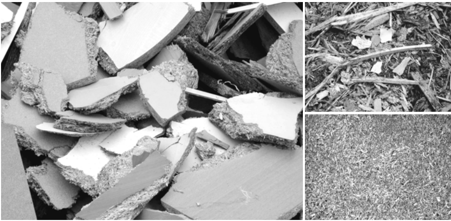
Fig. 5 Palm-sized pieces (approximately 5-10 x 10-20 cm) of particle boards (upper photo) as obtained from pre-crushing in the thermo-hydrolytic Conti-Recycling-Process of the Pfeleiderer Holzwerkstoffe & Co. KG (compare Fig. 4 and 6). Upon thermo-hydrolytic disintegration, sieving separates chips of intended sizes of 0.1 to 20 mm (lower panel right) from those that are too large and from other contaminations (upper panel left)
