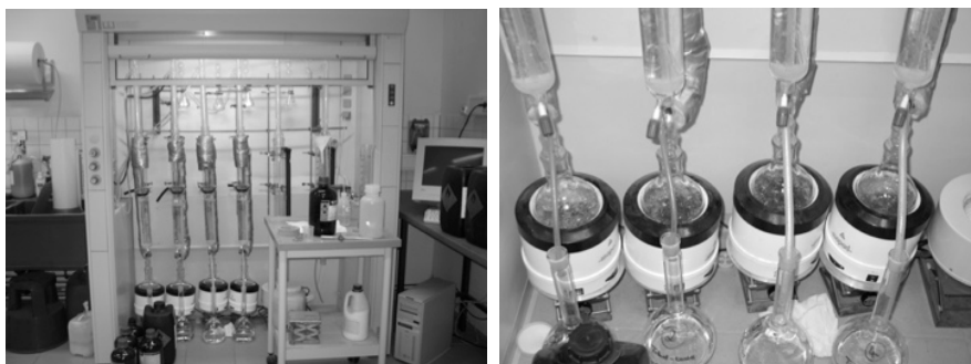
Fig. 14 Overview and detailed view of perforators in the chemical laboratory of the “Biotechnikum” at the Institute of Forest Botany in Göttingen used to measure formaldehyde emission of wood based panels according to European standard EN 120 (1993). Samples of fixed sizes (25 mm x 25 mm) are given into round bottom flasks, filled up with 600 ml of the solvent toluene, and boiled up in order to collect the formaldehyde in 1000 ml distilled water filled into the perforator elements attached to the round bottom flasks. After boiling for 2 h, the distillates are harvested from the perforator elements, mixed in appropriate volumes with acetyl-acetone and ammonium acetate, and incubated for 1 h at room temperature in the dark. The formaldehyde in the distillates will react with acetyl-acetone and ammonium acetate to form the yellow, strongly fluorescing 3,5-diacetyl-1,4-dihydrolutidine derivative. The concentrations of the 3,5-diacetyl-1,4-dihydrolutidine derivatives are measured in a photometer at a wave length of 412 nm and used to calculate the formaldehyde concentration in the original samples
