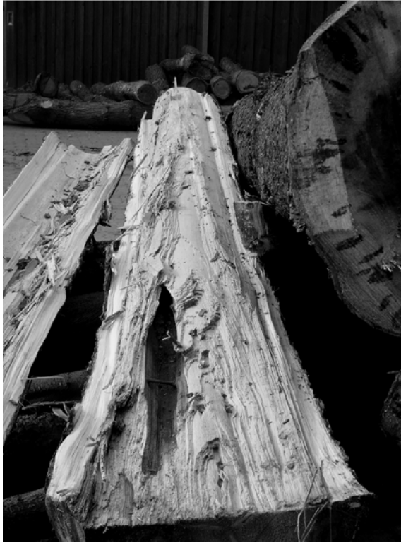
Fig. 10 Development of the fungus within the trunk. The lower 3 m of a felled stem of spruce have been trimmed due to an advanced decay by Heterobasidion . With the exception of the small outer sapwood ring, all interior wood is light-brownish stained due to the fungal infestation. By the advanced progress of decay, the outer sapwood was easily lifted from the decay column of the inner heartwood
