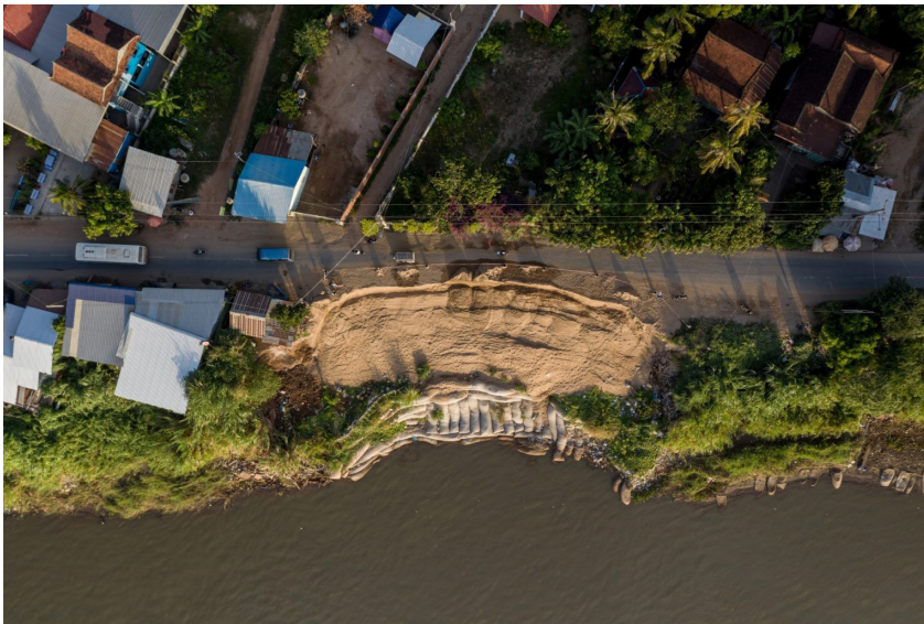
Abb. 5: „The aftermath of a riverbank collapse along the National Road No. 70A that occurred in Roka Koang in November 2021“ (Flynn and Srey 2022). © Andy Ball/University of Southampton.
