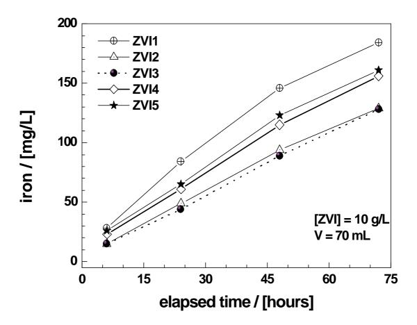
**Figure 1**: Comparison of the iron dissolution rate by the tested ZVI materials for 72 hours. ZVI1 is the scrap iron. The represented lines are not fitting functions, they just joint the points to facilitate visualization. The regression parameters (a and b) are listed in Tab. 3.
