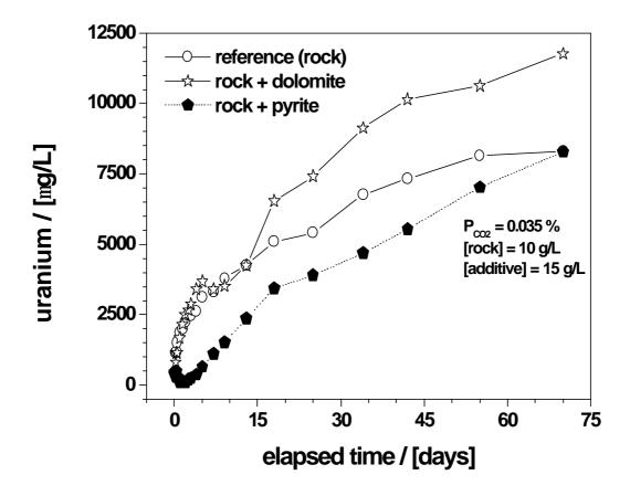
Figure 2: Impact of dolomite and pyrite on the evolution of uranium concentration as function of time in an air homogenized batch experiments for 70 days. Uranium is leached from a natural rock as described in ref. 36.  $P_{CO2}$  is the atmospheric partial pressure of  $CO_2$  (open system). The particle size of used materials was:  $0.315 \le d$  (mm)  $\le 0.63$ . The represented lines are not fitting functions, they just joint the points to facilitate visualization.
