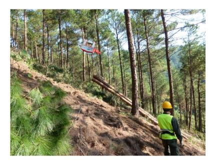
**Figure 4.** Recently introduced mobile standing skyline cable yarding extraction of long wood within a thinning demonstration for valuable saw log production at the Experimental Centre for Tropical Forestry in Pingxiang/Guangxi (Hoffmann, 2016).
