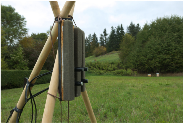
Figure 1. Setup used for testing microphone attachments outdoors. Foam strips reduced ultrasound echoes and the microphones were approximately 1 m above the ground and parallel to each other.
