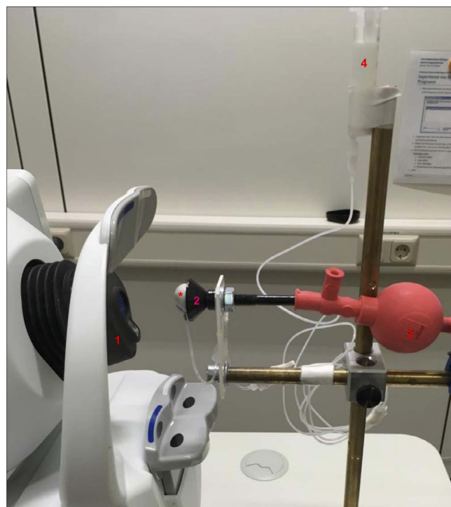
FIGURE 3. Experimental setup for ex vivo porcine eye scans. The OCT device was equipped with an add-on lens (1). The eyeball (asterisk) was placed in a custom-made funnel (2). Slight suction from a pipetting ball (3) kept the eye attached. The eye's anterior chamber was perfused through an open infusion system (4).
