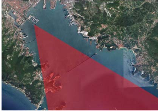
Fig. 13. Example application: tracking boats and ships using marine X-band radar. Aerial image of harbour, with sensor’s field of view shown in red.
