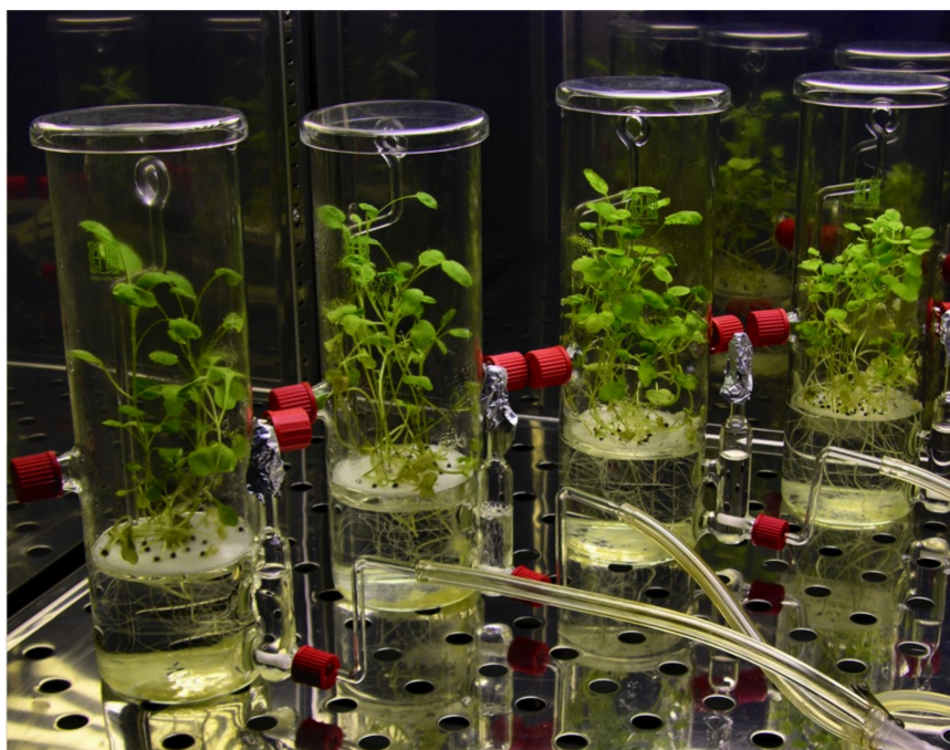
Figure 3. Oilseed rape ( Brassica napus L.) grown in sterile hydroponics. Ten plants per bioreactor were grown in 0.5× MS medium for three weeks at 24 °C with 12 h light per day. External light-shielding cylinders were removed for the photography.
