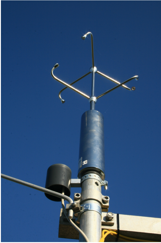
Figure 2. Low-cost eddy covariance instrumentation, featuring a uSONIC-3 Omni sonic anemometer and a BME280 thermohygrometer. The thermohygrometer is placed in a ventilated PVC housing below the sonic anemometer.
