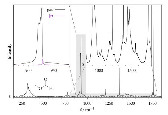
**Figure 1.** Gas-phase Raman spectrum of methyl methanoate. Left inset: Enlarged part of the ester linkage stretching mode  $v_{14}$  (vide infra) in comparison to a jet cooled spectrum scaled to be part of the gas phase spectrum. Right inset: Enlarged view of the baseline, which does not drop to 0 due to thermal excitation.
