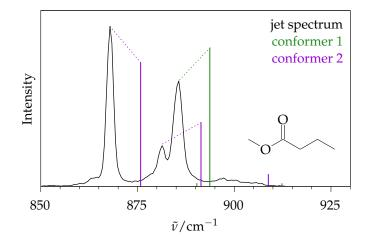
**Figure 2.** Enlarged part of a Raman jet spectrum of methyl butanoate (line) and calculated harmonic Raman spectrum for its two main conformers (vertical bars encoding predicted wavenumber and integrated intensity). Although a qualitative assignment is directly possible by implying a systematic anharmonic downshift, a quantification by signal integration is not, because the baseline does not drop to zero between the signals.
