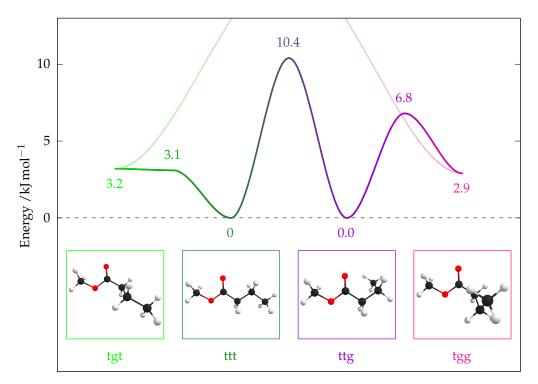
**Figure 9.** Relative energies and barriers of interconversion of the main conformers of methyl butanoate on CCSD(F12\*)(T\*)//B3LYP level (ZPE included). Isomerisation about the  $C_{\alpha}C_{\beta}$  bond is more feasible if the OCC<sub>\alpha</sub>C<sub>\beta</sub> dihedral is in t orientation (the barrier for g orientation exceeds the displayed energy range).
