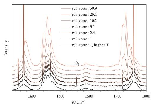
**Figure 3.** Raman jet spectra of methyl methanoate for widely different ester concentrations, scaled to the peak monomer signal at  $1755 \text{ cm}^{-1}$ . The expansion conditions are identical, except for the lowest trace, where a reduced distance to the nozzle (0.5 mm) leads to higher temperature. The O<sub>2</sub> signal is due to air impurity. The relative concentration of 2.4 was chosen for further analysis (bold trace).
