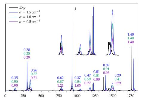
**Figure 7.** Black trace: Experimental jet spectrum of methyl methanoate. Coloured traces: rovibrational simulations for different Gaussian widths, matched to the strongest peak at 928 cm<sup>-1</sup>. In order for the calculated peak height of a vibration to match the experiment, the intensity of the simulated spectrum has to be multiplied with the numbers given.
