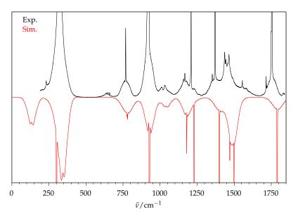
**Figure 6.** Experimental gas phase spectrum of methyl methanoate (**top black trace**) and rovibrational simulation for 298 K and  $\sigma = 1.0 \text{ cm}^{-1}$  (**bottom red trace**).
