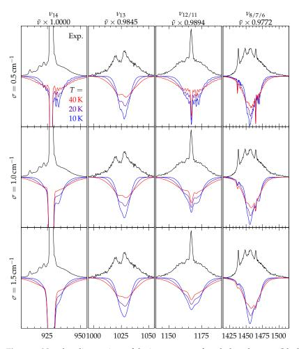
**Figure 5.** Near-baseline sections of the jet spectrum of methyl methanoate (black trace) and rovibrational simulations for different temperatures *T* and Gaussian widths  $\sigma$ . Calculated wavenumbers are scaled by the factors provided below the vibrational labels and calculated intensities are scaled to match the integrated experimental intensity.
