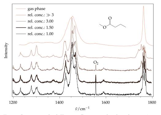
**Figure 10.** Raman spectra of methyl butanoate. Top trace: gas phase. Lower four traces: jet spectra with identical conditions, except for varying ester concentration.  $O_2$  and  $H_2O$  signals at 1556 and 1590 cm<sup>-1</sup> are from air impurity.
