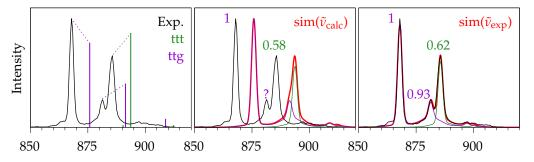
**Figure 12.** Jet spectrum of methyl butanoate (black, Figure 11, trace (e)) and three differently simulated spectra. **Left**: Raman cross sections indicated by vertical bars like in Figure 2. **Middle**: Rovibrational simulation, using calculated harmonic vibrational wavenumbers. The question mark indicates the inability to quantify the weaker ttg signal due to overlapping simulated band contours. **Right**: Rovibrational simulation, based on experimental vibrational wavenumbers.
