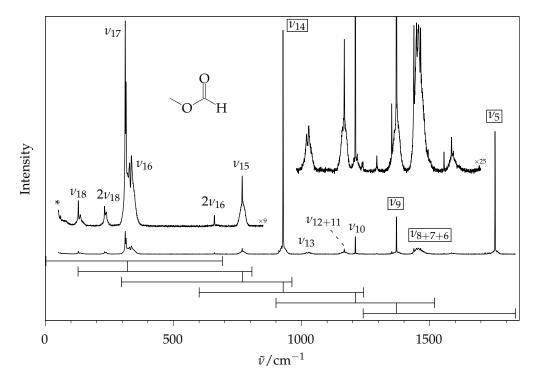
**Figure 4.** Experimental jet spectrum of methyl methanoate, constructed from six overlapping segments (horizontal bars, intensity matching at the vertical connection lines). \* marks air impurities, any signal  $<50 \text{ cm}^{-1}$  is distorted by a Rayleigh edge filter. The band labels  $v_5 - v_{18}$  ignore symmetry, see Table 1 for the associated dominant vibrational character and symmetry. Signals that are used for normalisation in Table 1 are framed.
