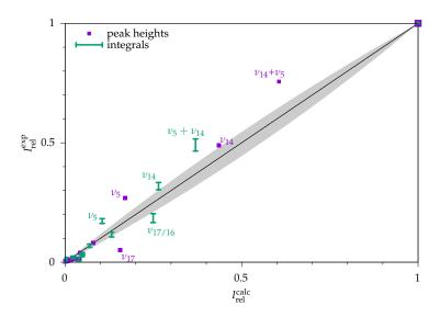
**Figure 8.** Ratio of calculated and experimental intensities for methyl methanoate. Violet points: peak height method ( $\sigma = 1.0 \text{ cm}^{-1}$ ). Green error bars: integral method; both normalised to give 1 in sum. Selected strong fundamentals and sums of fundamentals are labeled to exemplify that the deviations between experiment and theory are often correlated among the two methods. The area that would be covered by an anharmonicity effect of up to 20% is shaded in grey.
